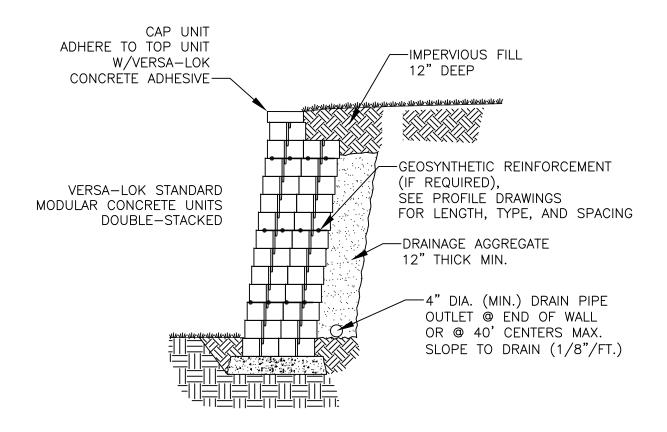
TYPICAL SECTION - DOUBLE-STACKED STANDARD UNIT RETAINING WALL
